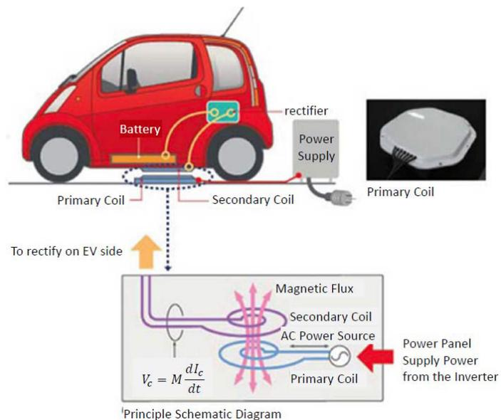
Figure 1. Schematic Diagram of Inductive Power Transfer System for EVs.
